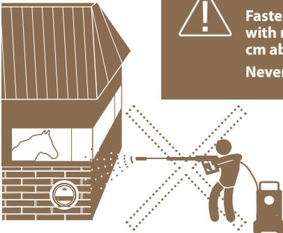
**Energizers must be installed in a dry place.**
