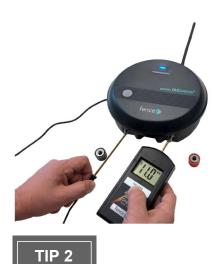
12 V battery power supply: LED flashes red > battery voltage is below 12 V, an acoustic alarm sounds if the battery voltage drops below 11.6 V. A minimum operating voltage of 12 V is suitable for operation, then the LED stops flashing red. Mains: power supply: LED does not flash or light > check the fuses and the main power distribution board
